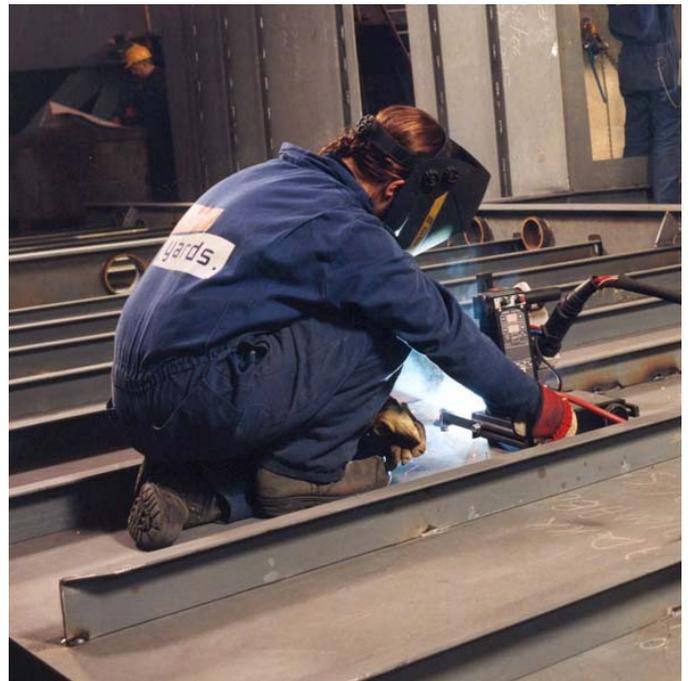
Cored-wire welding - a process in keeping with the times
