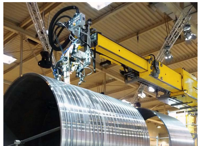
External welding with Telbo™
