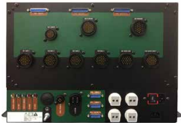
Amplifier and control enclosure
