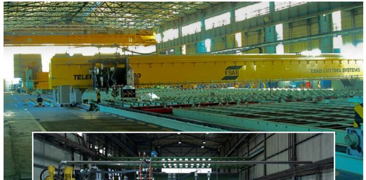
The integrated ESAB cutting automation solution improves weld quality throughout the yard by providing more consistent edge preparation.
