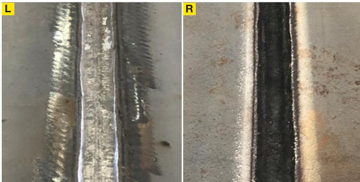
Notice the perfect reinforcement level on top side of the bead **L** and excellent the back side bead **R** profile.
