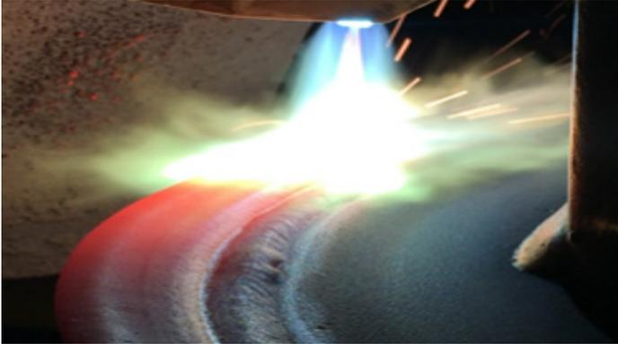
ESAB's Italian Application Engineering team provided onsite feedback to EWAC team in India. Working together they created a modified powder formulation — a blend of self-fluxing nickel alloy (NiCrBSiB) + 60% tungsten carbide — that met all of the olive oil equipment manufacturer's needs.
