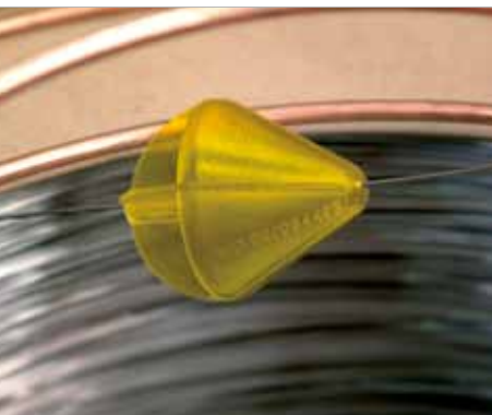
The pear is an ESAB invention that facilitates a smooth transition when the wire crosses over from one drum to the other. The wire passes through the pear which is placed on top of the first drum when it is installed. When the drum is empty, the pear crosses over while the wire conduit swings to the new drum.
