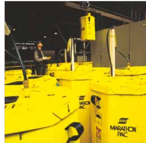
Marathon Pac™s are easily lifted to the welding station using the special yoke.
