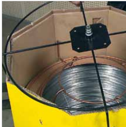
Step 2. Place the wire conduit attachment or "spider" on top of the Marathon Pac™.
