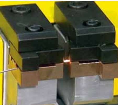
The wire from a second Marathon Pac™ is joined to the first using a special portable butt welding device.
